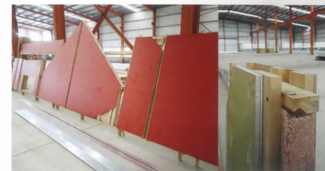
Mock-up of decorative high-pressure laminated panels 高压装饰层积板大样
